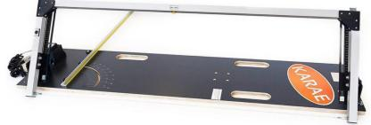
Widely used by everyone from Sculptors to Roofers. It is ideal for cutting Styrofoam and Similar synthetic insulating materials.
