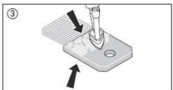
③ On one side, fuse the stainless-steel mesh into the plastic. Heat the mesh all over and fuse by applying even pressure.
