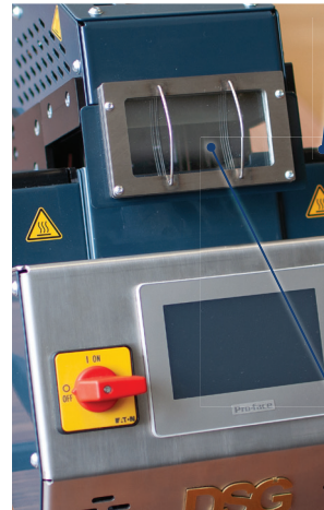
Capacitive sensor for process launch and cycle count.
