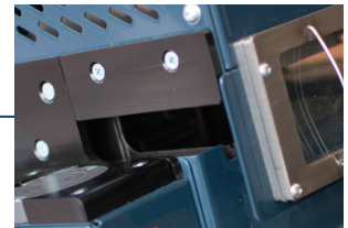
Infrared quartz heating elements covering 270° circumference with up to 530°C.
