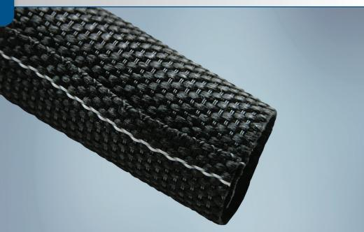
**ROUNDIT®** 2000FR is a wrap-around sleeving manufactured from flameretardant polyester monofilaments and multifilaments, designed for mechanical protection and maintenance of wire and cable bundles. Its construction with 100% covering ratio provides good abrasion resistance.
