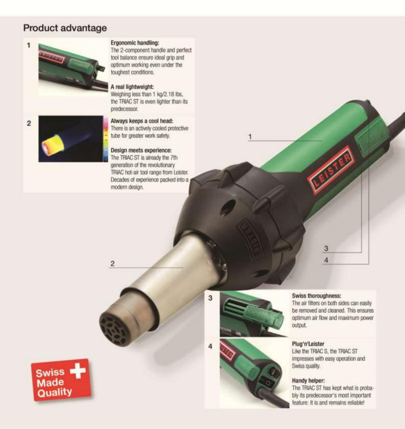
perfect weight balance. The innovative motor and turbine design, combined with the heating element familiar from the TRIAC AT, enhance the value even more. The two air filters that can easily be removed and cleaned are also new. More than 80 nozzles fit onto the TRIAC ST; these are also compatible with the TRIAC AT and TRIAC S. That makes all conceivable applications possible, both indoors and outdoors.
