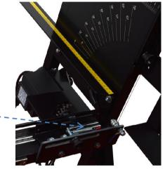
**Caution 1:** Excessive power output and heat generation may cause the damage to the tansformer. Use only the power output for proper cutting. The wire does not need to be red hot to move through foamed plastics.
