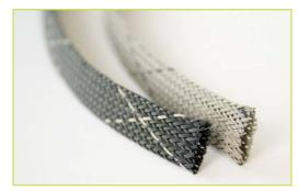
**Harnesses** - Hilflex PG FR is used extensively as a harness sleeve, the open construction of the braid allowing branch terminations to be made through the sleeve wall, which greatly speeds manufacture.
