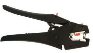
Powerful, heavy duty wire and cable stripper capable of handling modern insulation wires and cables up to 16mm2 . The tool is constructed from glass filled polyamide for strength and lightness with steel liners or added rigidity.
