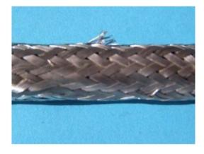
NOT ACCEPTABLE Damaged and nicked conductors
