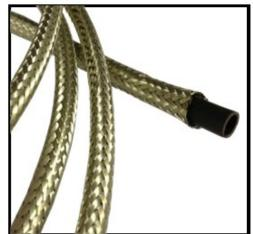
6, When all of the Braided sleeving is fed onto the cable remove the former and paper tape.
