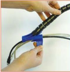
2. Place the HILZIP PPT onto the mounting tool.
