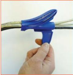
1. Using the special mounting tool, insert the cable loom.
