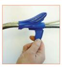
1. Using the special mounting tool, insert the cable loom.
