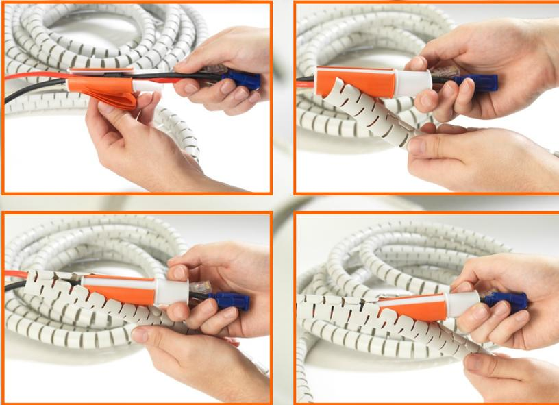
Hand tool supplied for quick and easy installation
