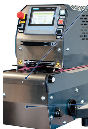
Siemens touch panel for quick monitoring of shrinking process and easy data input
