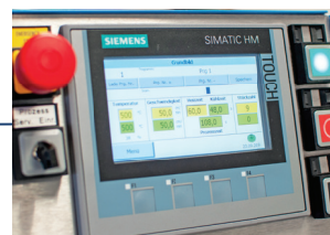
Siemens touch panel for quick monitoring of shrinking process and easy data input
