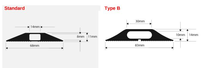
Profiles are designed to house one or more cables in a variety of combinations depending on the application, allowing the user total flexibility to secure a wide permutation of lead and cable sizes. "Snap" open the membrane in the base of the profile, push in the cable and lay the protector in place.
